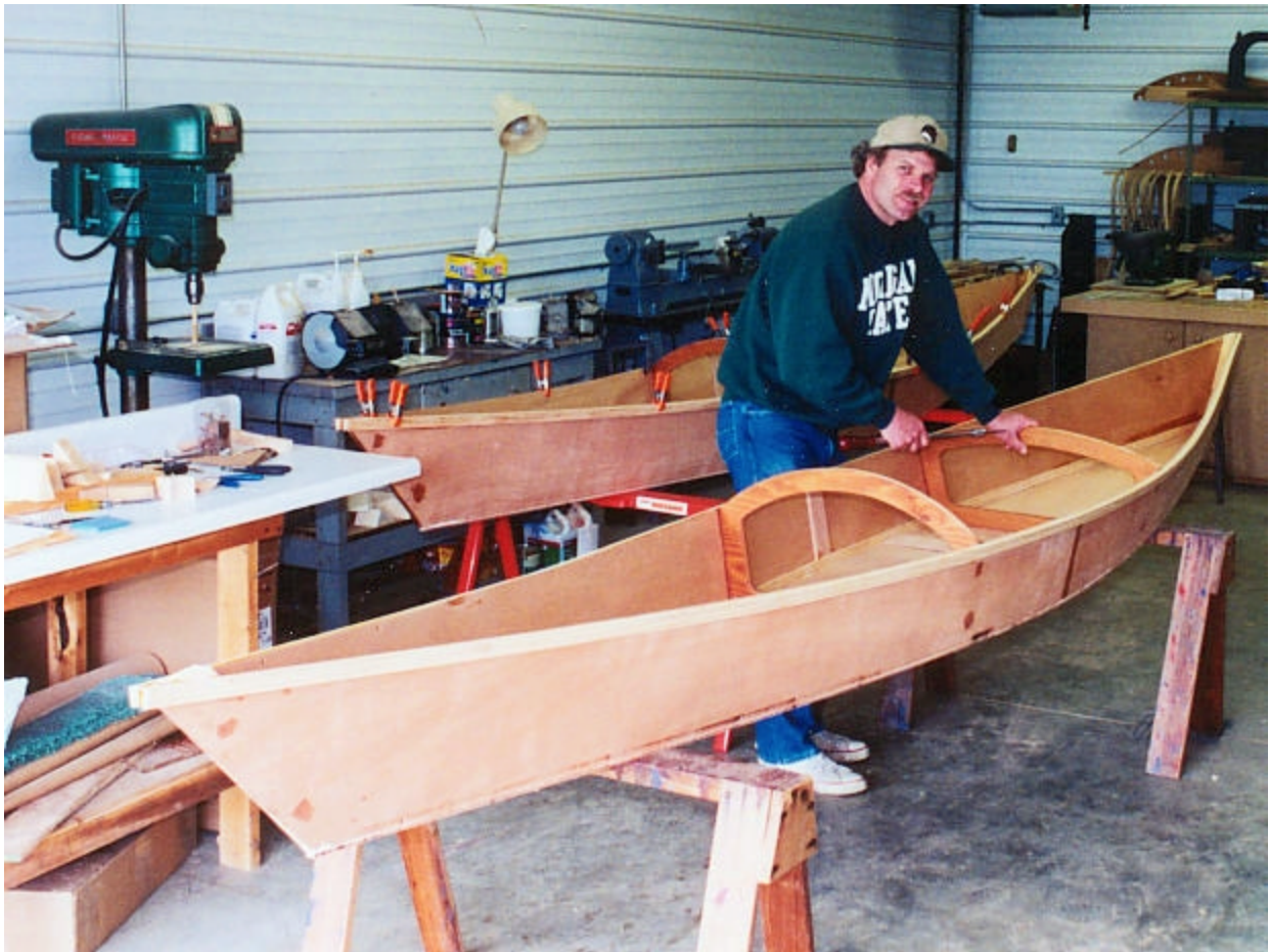
Professional boatbuilder Scott Gearhart sets two frames in place in JOZEBOTE. NEP eliminates the need for molds, strongbacks, building jigs or fixtures. Building can be done anywhere on two saw horses.
