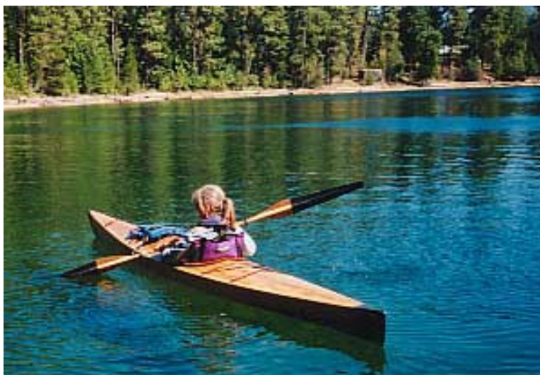
Donna Hime taking a paddle in the Paul Butler built 15' epoxy plywood kayak. The black is graphite epoxy used as scruph barrier protection.
